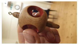
To finish, Dave turned the two finials, and they are fitted into the 6mm holes at top and bottom of the finished piece.
