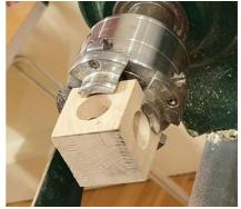
Next, drill a 6mm hole into the end grain through the centre. This will be used to take a mandrel to finish turning it.
